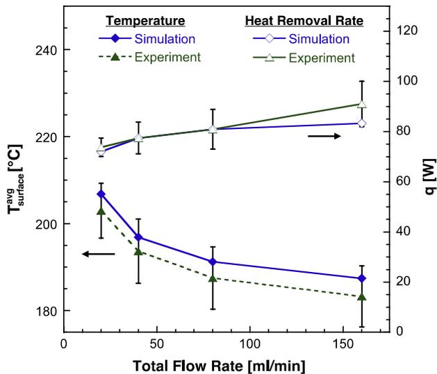
**Fig. 13.** Average top surface temperature ( $T_{avg\ surface}^{avg}$ ) and heat removal rate ( $q$ ) as a function of total flow rate compared for the model and experimental results at an environmental temperature of 325 °C. Results are shown for the MPC specimens. Error bars for experimental data represent one standard deviation. (For interpretation of the references to color in this figure legend, the reader is referred to the web version of this article.)
