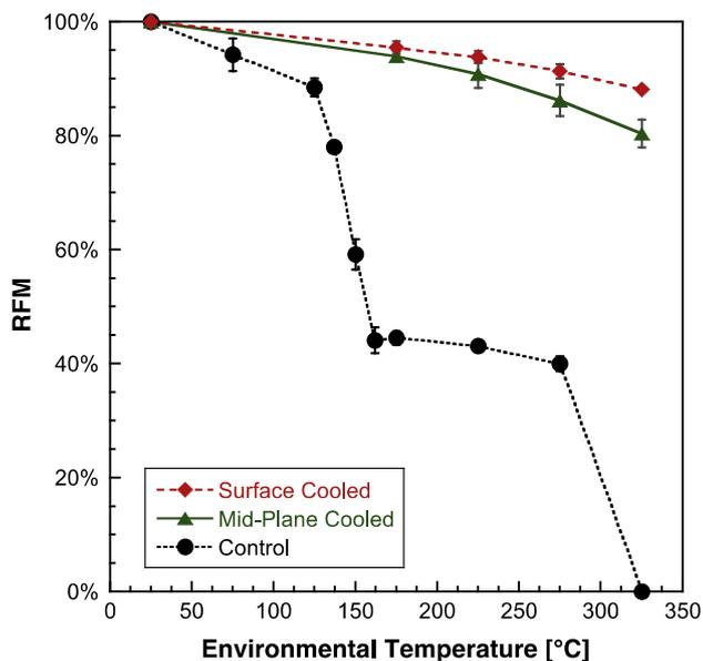
**Fig. 6.** Retained flexural modulus (RFM) as a function of environmental temperature. Control specimens (no microchannels) were thermally degraded at 325 °C and retained no flexural capacity. Vascular specimens were tested with a coolant flow rate of 160 mL/min. Error bars represent one standard deviation. (For interpretation of the references to color in this figure legend, the reader is referred to the web version of this article.)
