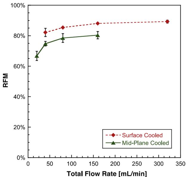
**Fig. 7.** RFM as a function of the total coolant flow rate in a 325 °C environment. Error bars represent one standard deviation. (For interpretation of the references to color in this figure legend, the reader is referred to the web version of this article.)
