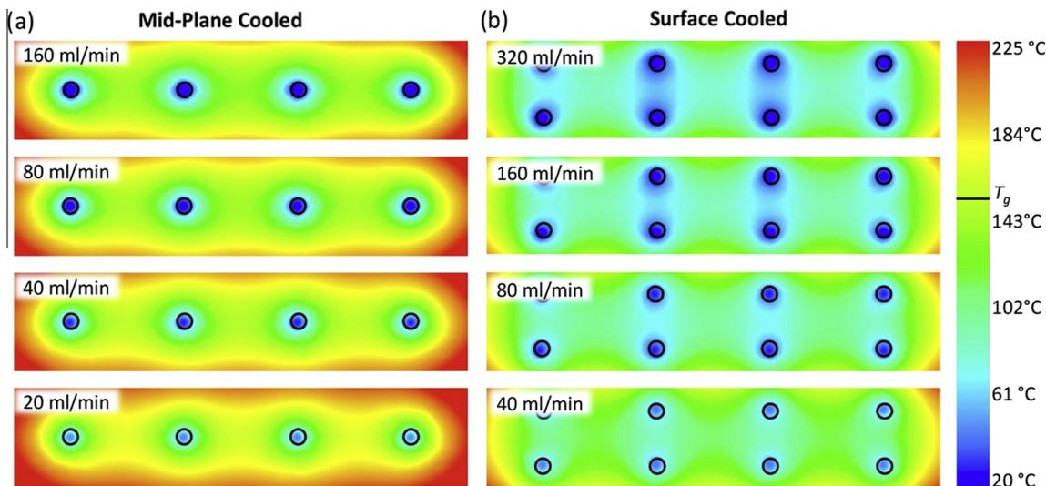
**Fig. 15.** Temperature profiles along the  $y = 50$  mm plane from simulation results for the MPC and SC samples in a  $325$  °C environment at each value of total flow rate tested during experiments.  $T_g$  is marked on the temperature map. The edge of each channel is marked by black circles. (For interpretation of the references to color in this figure legend, the reader is referred to the web version of this article.)
