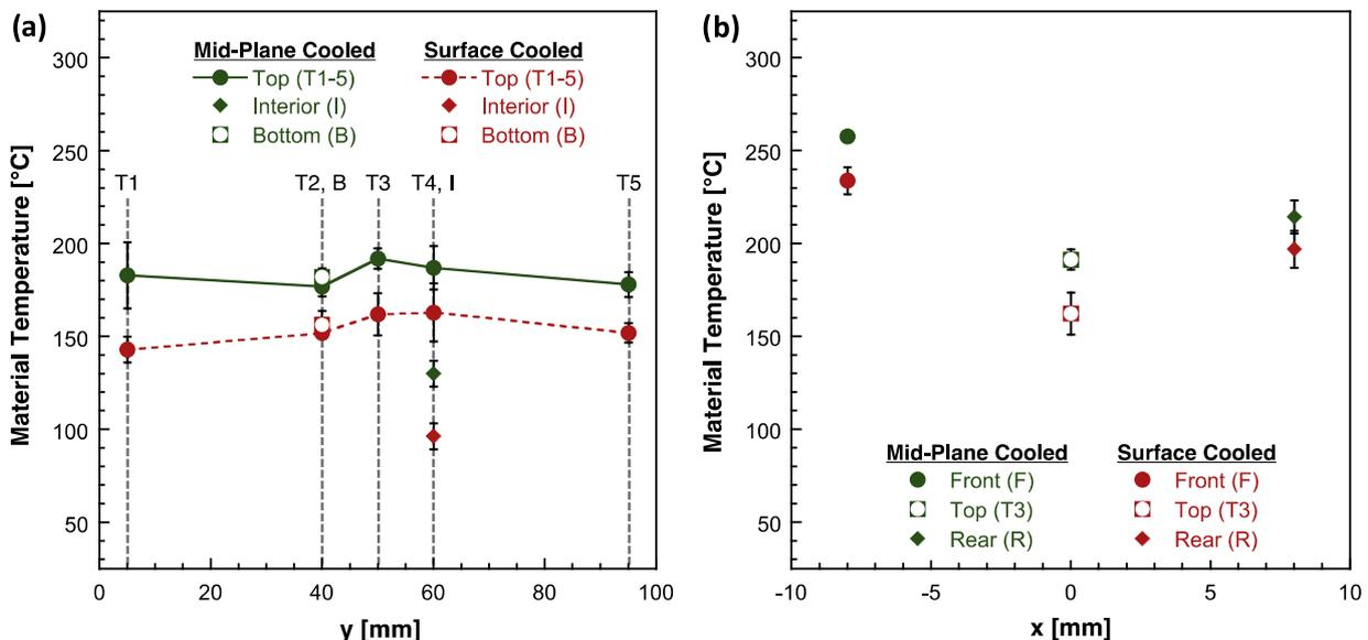
**Fig. 9.** Temperature distribution for actively cooled specimens. Temperature (a) along the  $x = 0$  plane and (b) along the  $y = 50$  mm plane for actively cooled composites in a 325 °C environment at a total flow rate of 160 mL/min. See Fig. 3 for detailed description of thermocouple location. Error bars represent one standard deviation. (For interpretation of the references to color in this figure legend, the reader is referred to the web version of this article.)
