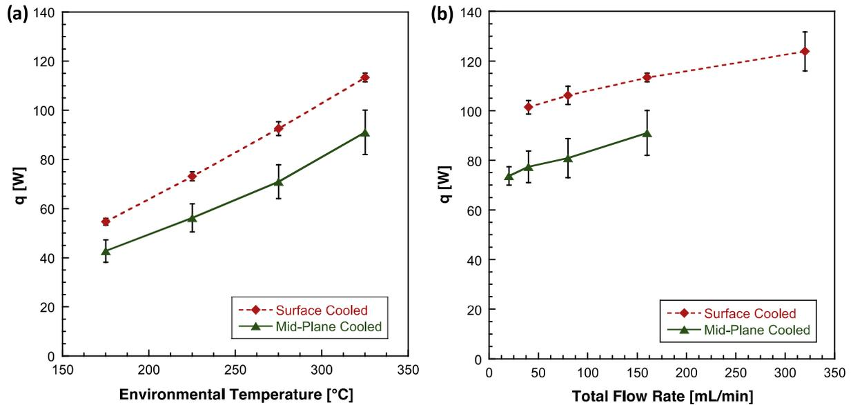
**Fig. 10.** Heat removal rate ( $q$ ) for vascular specimens for all testing conditions. (a) Heat removal rate as a function of environmental temperature for a fixed total flow rate of 160 mL/min. (b) Heat removal rate as a function of total coolant flow rate for a fixed environmental temperature of 325 °C. Error bars represent one standard deviation. (For interpretation of the references to color in this figure legend, the reader is referred to the web version of this article.)
