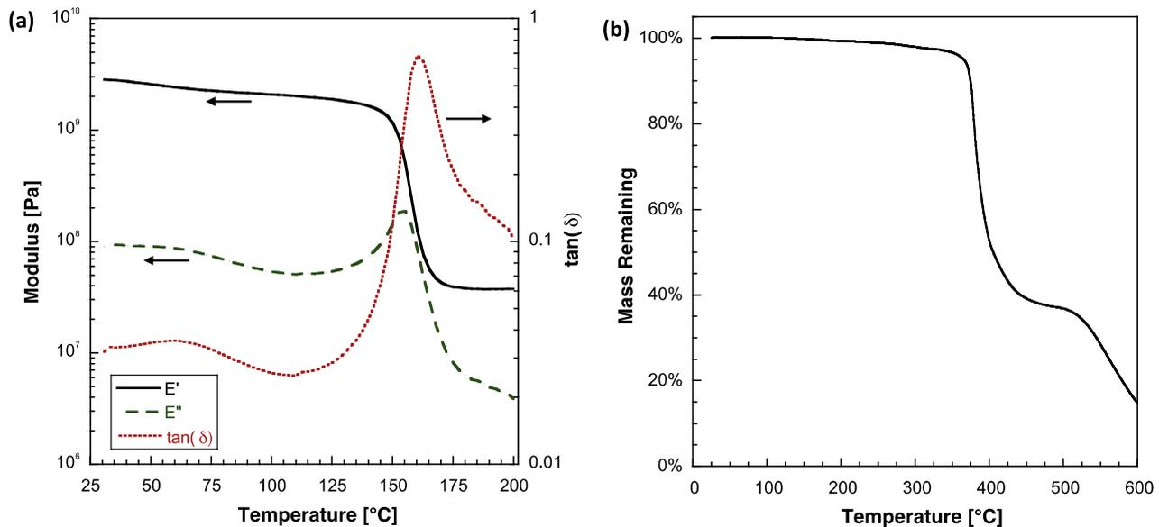
**Fig. 5.** Thermal and mechanical characterization of the epoxy matrix. (a) DMA testing results showing the storage modulus ( $E'$ ), the loss modulus ( $E''$ ) and  $\tan(\delta)$ . (b) TGA testing results in an air/nitrogen environment (flow rates of 35 mL/min for each). (For interpretation of the references to color in this figure legend, the reader is referred to the web version of this article.)
